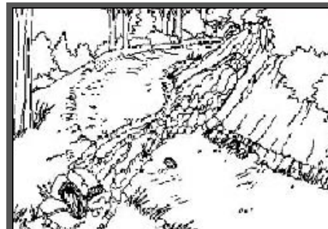
Figure A2. Road maintenance is needed to maintain roadway surface drainage patterns and remove slides that block ditches and culvert inlets.
